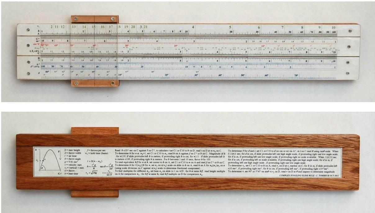
Fig 2 Complex Slide Rule, front and back.
